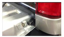
**Tech Note:** For certain truck models, the adapter ring may be needed to provide optimal fit and theft deterrence. The adapter ring needs to be slid over the passenger side hinge before completing Step 3.
