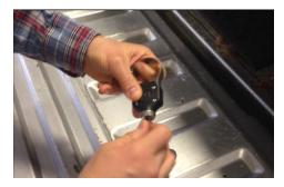
3. Place the metal hasp around the passenger side hinge of the tailgate. See photo below.
