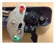
Install the return spring onto the plastic lock housing. Start by inserting one leg of the spring into the housing. Grab the spring from the outside diameter and turn clockwise till you can insert the other leg of the spring into the housing. Both legs must be fully seated down in the half shape moon cut out
