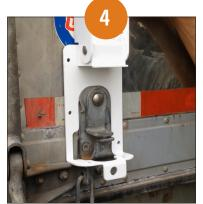
Remount the Seal Safe and align with stencil marks.
