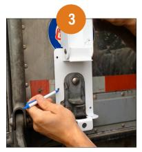
Trace the outline of the Seal Safe and hole pattern (a pencil will work best). Remove Seal Safe. Drill the holes that were stenciled to accept the 1/4" rivets or fasteners.
