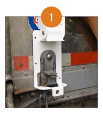
While facing the trailer at the back of the truck, open the right door handle. With the Seal Safe cover raised, place the Seal Safe over the latching mechanism.
