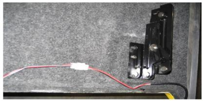
7) If using the in cab remote button option, route the Button Harness into the cab of the truck through an existing grommet. Drill a 1/2" hole in the desired location of the button and mount it through the hole. Attach the black wire to a good ground and plug the gray wire from the Button Harness into the gray wire on the Truck Harness.
