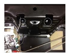
**STEP 2** - Remove the handle rod from mechanicals by turning the green rod clip and pulling the rod out of the clip. Swing the rod up and out of the way. Remove the two screws holding the factory handle in place; there are tabs that will hold the handle from falling out of the tailgate, but for extra assurance hold the handle in place so not let the handle to fall. Remove the factory handle.
