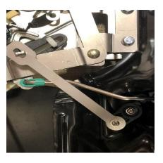
**STEP 5** – Install the crank linkage by holing the slotted end onto the bolt linkage and then screw the black locking pawl onto the key cylinder using the provided screw, split lock washer, and flat washer.
