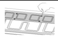
**STEP 1:** Remove the access panel from the inside of the tailgate. (Remove the bedliner cover if applicable)
