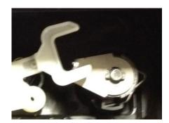
**Step 3:** Install the power lock assembly. Start by removing the handle mounting bolt on the passenger side of the handle. Position the power lock assembly so that one hole is over the plastic stud and the other is over the mounting bolt hole. The arm on the slide bar should be positioned between the white plastic locking toggle and near the arm of the cam, as shown in picture 4. Reinstall the bolt and tighten.
