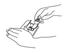
**5.**Lift the handle and insert the POP&LOCK with the lock in the unlocked position.
