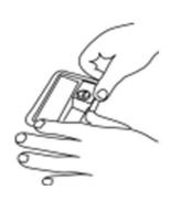
**7.**Push the black plastic insert in fully and tighten the mounting screw.
