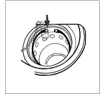
Secure fuel cap chain to the pre-inserted interior ring as shown in the diagram.
