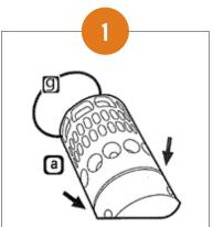
Apply black rubber gasket (g) to the outside of the Diesel Defender (a). The gasket should fit into the indented ring adjacent to the set-screw holes.
