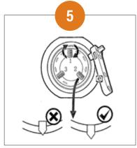
With an optional 1/8" allen wrench or the included toolkit (e), carefully tighten the screws to securely mount the Diesel Defender into the neck of the fuel tank. Be careful not to loosen the set-screws or drop any toolkit accessories into the fuel tank during installation. Tighten set-screws until they are no longer visible within the interior diameter of the Diesel Defender.
