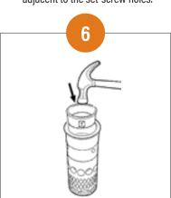
Insert interior cover ring (f) into the inside diameter of the Diesel Defender and tap into place with a hammer.
