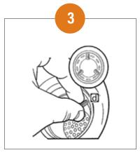
Insert set-screws (d) into the 3 interior holes near the top of the Diesel Defender and tighten by hand not to exceed outer diameter.
