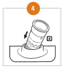
Insert the Diesel Defender (a) into the neck of the diesel fuel tank.
